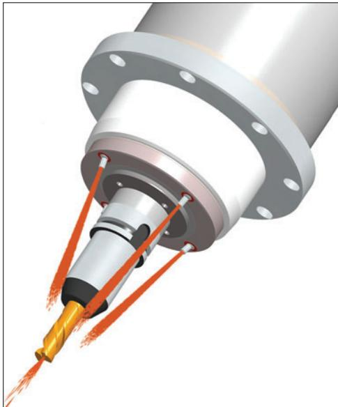
For coolant through the spindle and the cutting tool **TDM** has designed internally a rotary union with most interesting performances. It allows to obtain a pressure of 300 bar up to 30'000 RPM. This peculiarity allows to drill in a short time deep holes also for small diameters. Moreover its special conception guarantees a much higher life in respect to traditional rotary unions.
